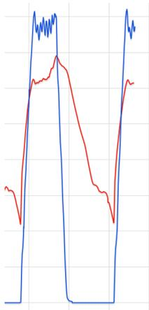
This chart shows how the nitrification / denitrification phase works. The red curve is the redox curve, the blue curve, the value of the dissolved oxygen in the wastewater. At the beginning of the aeration, the oxygen value increases, which from a value of 2 mg / l O<sub>2</sub>
